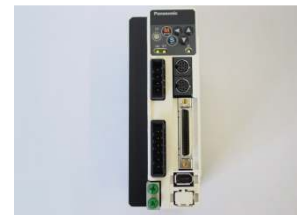
4. SP 006 732 DRIVER, ROLLER DRIVE SERVO
