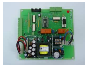
3. SP 006 474 PCB, CONVEYOR CONTROL
