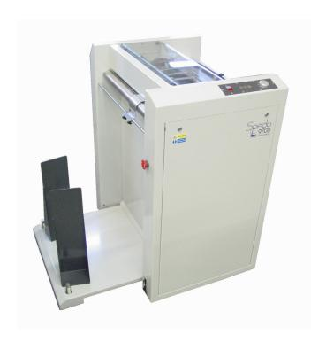
The SPEDO 9700 SLITTER MERGER is used to centre split stationery and merge forms prior to sheeting with a Spedo cutter.
