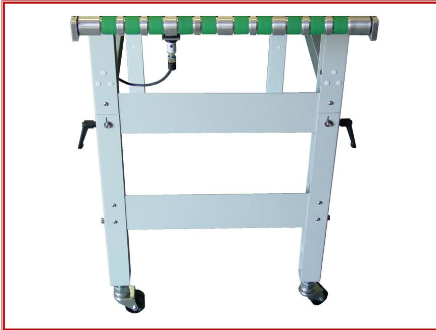
Fig 1.2 Fitting the front leg assembly.
