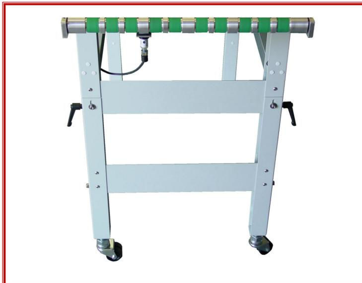
Fig 1.8 Releasing the conveyor height locking levers.
