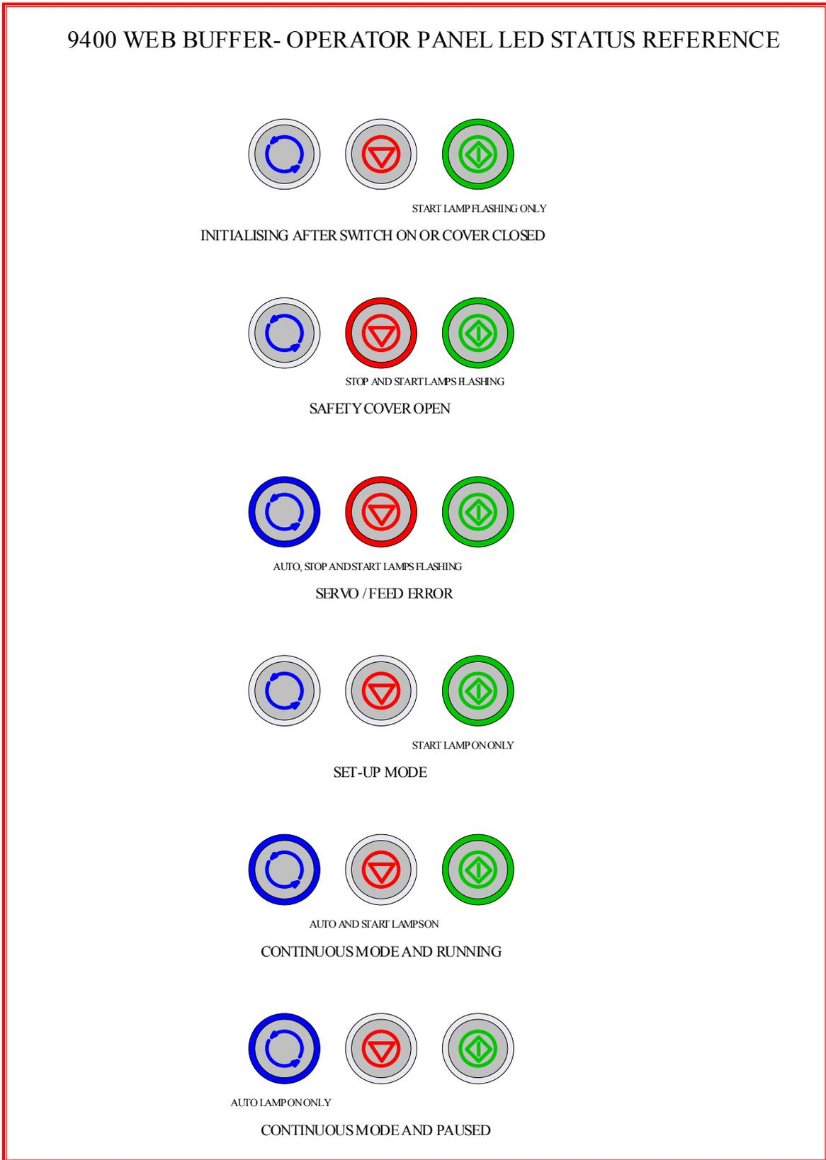
**Fig 1.4 Operator LED status explained.**
