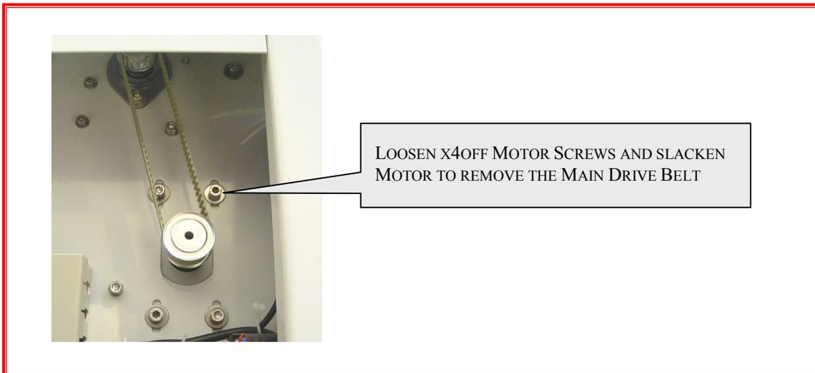
Fig 1.7 Removal of Main Drive Belt
