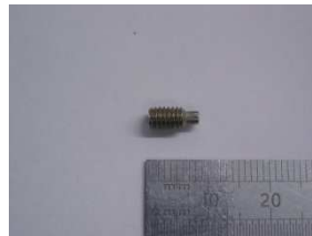
15. SP 000 378 SCREW, M4 x 8, DOG POINT GRUB
